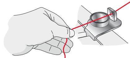
*Note: When using decorative threads, place the thread unreeling disc as shown to prevent the thread from getting caught on the edge of the spool.*
