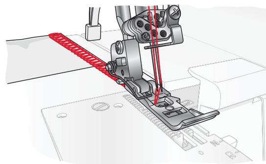
*Tip: When you have re-threaded the machine, always chain off and test sew a sample to test thread tension.*
