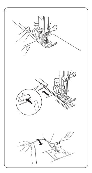
Raise the presser foot and position the fabric next to a stitching guide line on the needle plate.
