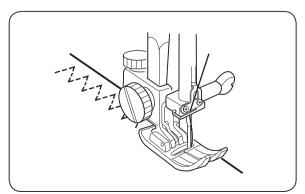
Place the fabric under the presser foot so that the edge will be slightly inside the right hand side of the presser foot.
