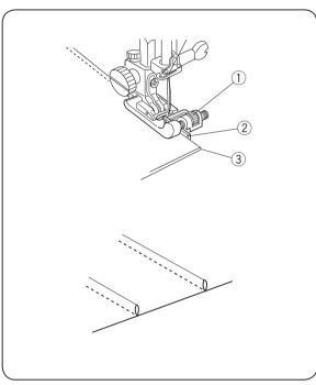
Fold a fabric wrong side together and Lower the needle into the fabric 0.1-0.2~cm~(1/16') inside the folded edge.
