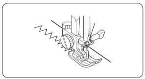
Simple zigzag stitch is widely used for overcasting, applique, sewing on buttons, etc.
