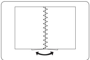
Sew seam and press seam allowance open. Sew pattern stitch on the right side of garment centering stitches over the seam line.
