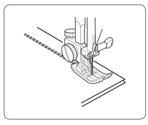
This strong, durable stitch is recommended where both elasticity and strength are needed to insure comfort and durability.
