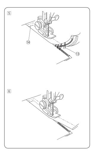
5 Raise and release the foot, and re-attach it with the left side pin.
