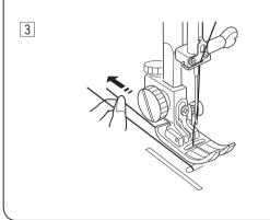
3 Pull 15 cm (6") of both threads back and under the presser foot.
