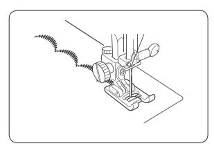
Sew a row of stitches and adjust the thread tension so the needle thread should appear on the reverse side of the fabric.
