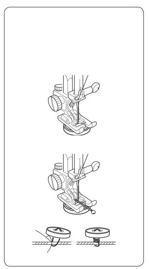
Tape the button over the placement mark. A pin can be placed on top of the foot to from a shank.
