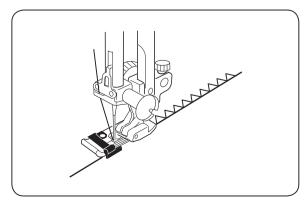
This type of stitch is used on the seam allowance to prevent fabrics from fraying at raw edges. It can be used to finish a hem edge. Place the edge of the fabric next to the black prong of overedge foot C.
