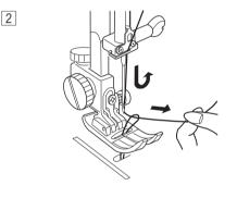
2 Turn the handwheel slowly towards you with your right hand until the needle goes down and continue turning handwheel until the take-up lever is at its highest position. Lightly draw up the needle thread forming a loop of bobbin thread.
