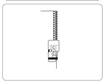
This stitch can be used for sewing fabrics that tend to fray extensively such as linens and gabardines. Two rows of zigzag stitches are simultaneously sewn over the edge to insure that your seams will not ravel. Adjust the thread tension so both the needle and bobbin threads meet at the edge of the fabric.
