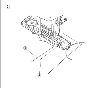
2 Start the machine and sew the buttonhole. Each side of the buttonhole and the bartacks will be sewn over the cord.
