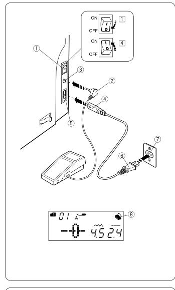
If you wish to use the foot control, insert the pin connector into the jack on the machine.
