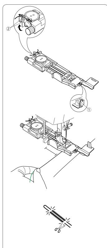
Place the button on the button holder on the buttonhole foot.
