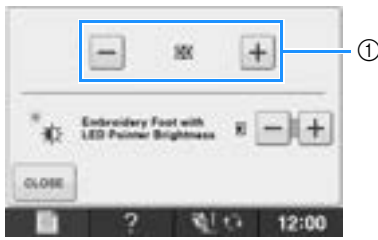
① LED pointer adjustment
