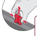
When removing the embroidery unit from the box for the first time, be sure the shipping brace on the underside of the embroidery unit has been removed.
