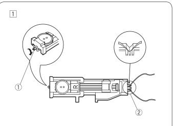
1 Use the same procedure as the square buttonhole sewing. Set the stitch width to match the thickness of the cord used.
