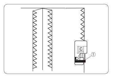
Place the fabric edge next to the guide on the foot and sew while guiding the fabric along the guide.
