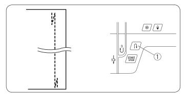
Use this stitch to secure the beginning and the end of a seam with backstitching.
