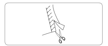
Place your fabric to allow a  $5/8^{\circ}$  (1.5 cm) seam. Trim excess close to the stitching. Be careful not to cut the stitches.
