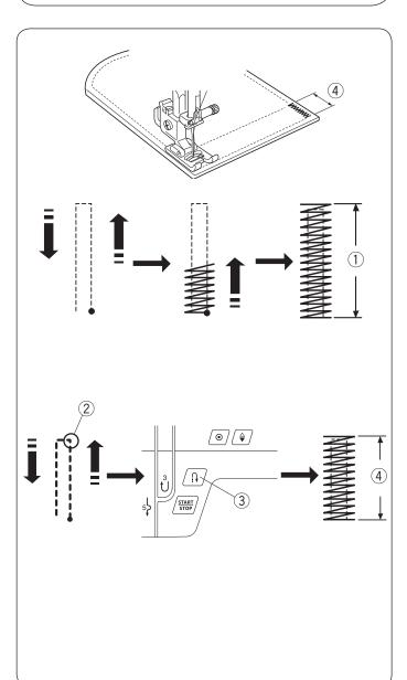
Tacking is used to reinforce pockets, crotches and belt carriers where extra strength is needed.
