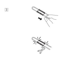
3 Pull the loose ends of the filler cord to tighten it.
