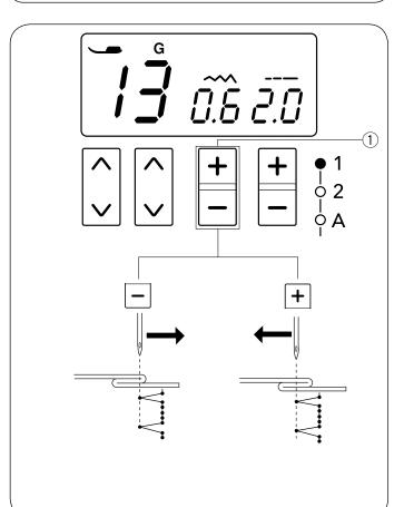
Adjust the needle drop position as follows:
