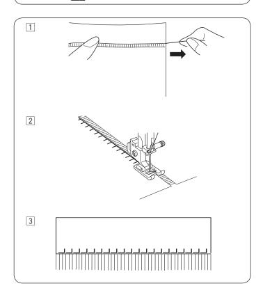
Fold the fabric with the wrong sides together. Place the folded fabric under the blind hem foot.
