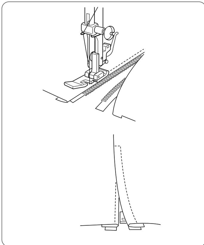
Pin or baste zipper tape to fabric and place it under the foot. Smooth the threads toward the back and lower the foot. To sew the left side of the zipper, guide the zipper teeth along the edge of the foot and stitch through the garment and zipper tape. Turn the fabric and sew the other side of the zipper in the same way as you did the left side.
