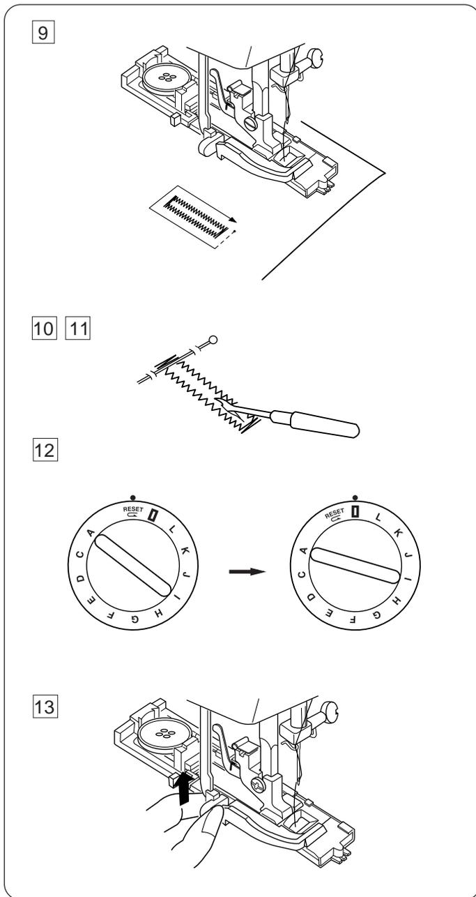
9 Sew slowly and stop the machine when a buttonhole is completed.
