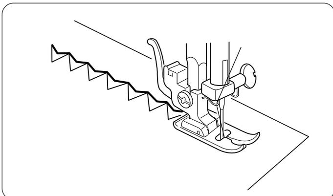
If forward and reverse feeds become unbalanced due to the type of fabric, adjust the balance by turning the stitch length dial as follows:
