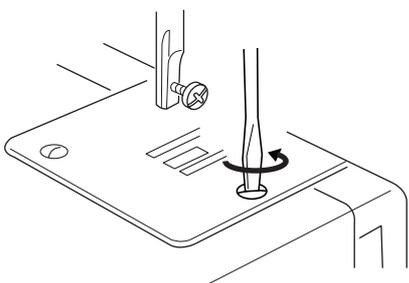
With a brush, clean out dust and lint clogging the feed dog teeth. Reset the needle plate.
