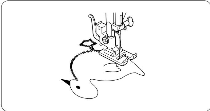
Baste (or fuse with iron-on fabric joiner) applique pieces on the fabric. Stitch around the applique making sure the needle falls along the outer edge of the applique. When sewing corners, lower the needle down into the fabric. Raise the presser foot and pivot fabric to the right or left.
