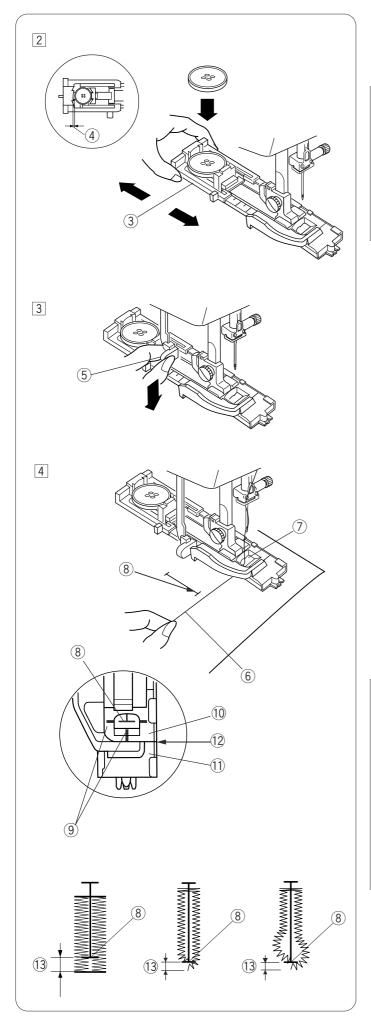
Pull the button holder to the back, and place the button in it. Push it together tightly to the button.
