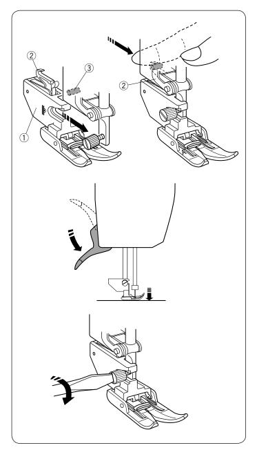
Attaching the Dual Feed Foot Attach the dual feed holder to the presser bar.
