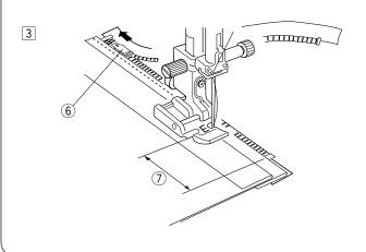
2 Attach the zipper foot E with the pin on the right hand side.
