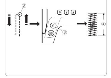
Tacking is used to reinforce pockets, crotches and belt carriers where extra strength is needed.
