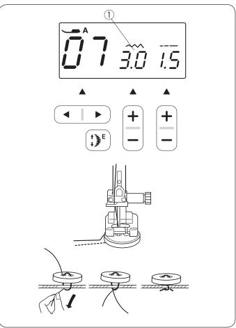
Lower the feed dog (refer to page 16). Set the speed control slider at a slower speed.
