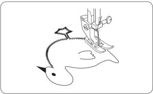
Baste (or fuse with iron-on fabric joiner) applique pieces on the fabric.
