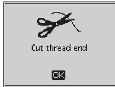
9. When the first color is completed, your machine stops. A pop-up message appears on the GraphicDisplay asking you to change color. Re-thread with the next color and continue embroidering by pressing Start/Stop. Each color segment is tied off at the end and the needle thread is cut.
