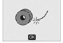
Remove any thread from under stitch plate and in bobbin area and press ok
