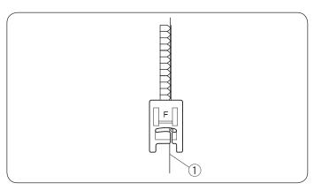
This industrial inspired overlock stitch is excellent for assembling and finishing fabrics together in one step. Apply ribbing to knits and garment retains its shape. Elna invented this stitch in 1982.
