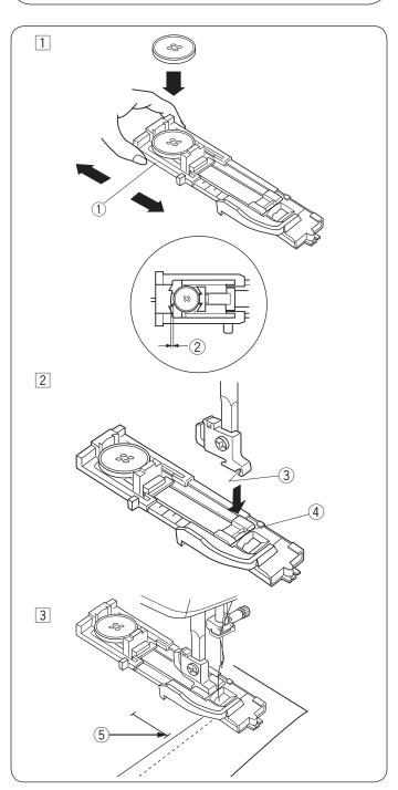
The size of a buttonhole is automatically set by placing a button in the rear of automatic buttonhole foot R.
