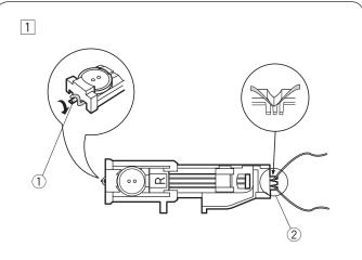
Use the same procedure as the square buttonhole sewing. Set the stitch width to match the thickness of the cord used.
