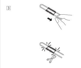
3 Pull the loose ends of the filler cord to tighten it.
