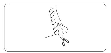
Place your fabric to allow a 5/8" (1.5 cm) seam. Trim excess close to the stitching. Be careful not to cut the stitches.
