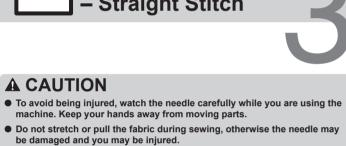
• Do not use bent or broken needles, otherwise you may be injured. • Take care that the needle does not hit basting pins or other objects during sewing. The needle may break and you may be injured.
