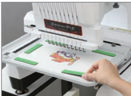
Secure with the magnets
