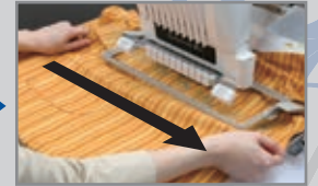
Simply slide the cloth and fit the frame
