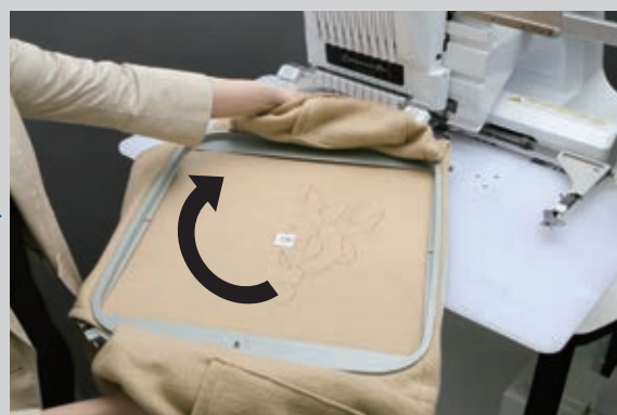
Rotate the frame when half the design is complete
