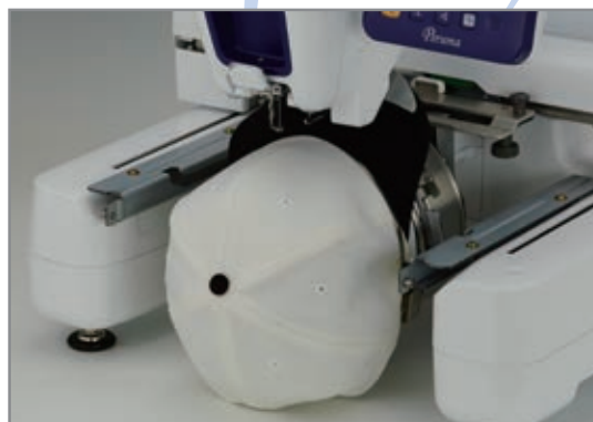
Set completed cap directly onto the machine
