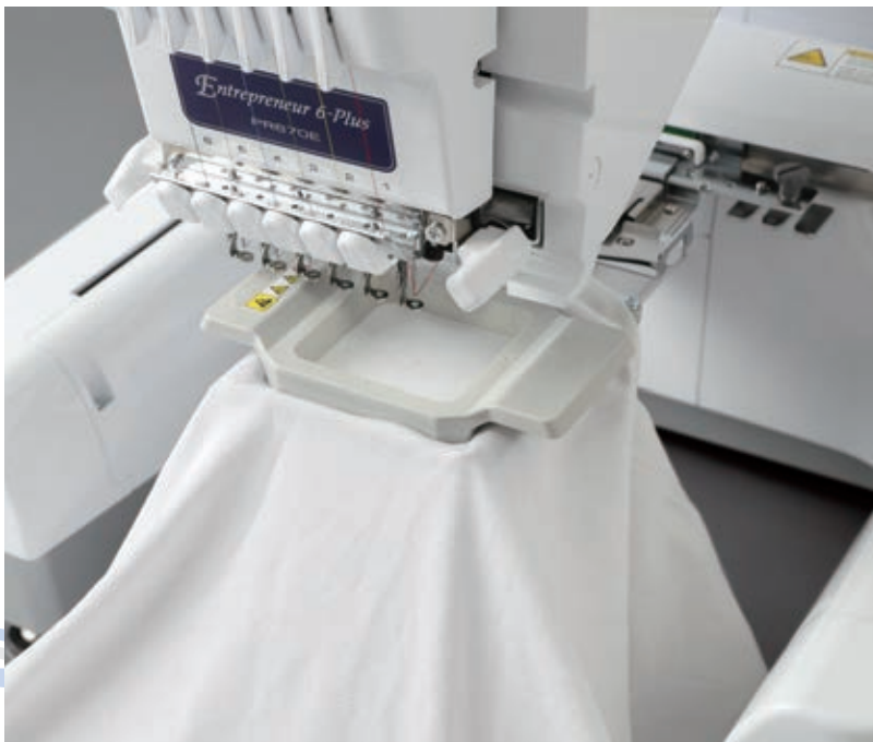
Simple framing, without tightening thumb screw.
