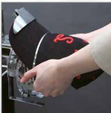
Stretch the cap over the frame
