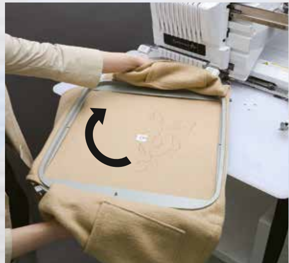
Rotate the frame when half the design is complete and embroider the rest of the design.
