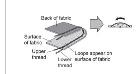
**Solution:** Reduce the tension by turning the upper tension control dial to a lower number
