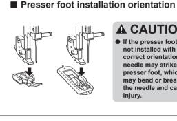
**▲** CAUTION If the presser foot is not installed with the correct orientation, the needle may strike the presser foot, which may bend or break the needle and cause injury.
