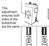
Turn the buttonhole fineadjustment screw with a large screwdriver as indicated in the illustrations, according to the buttonhole appearance.
