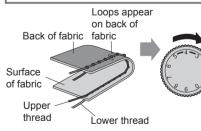
Solution: Increase the tension by turning the upper tension control dial to a higher number.
