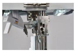
> Tighten the needle screws.
