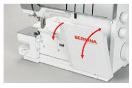
> To close the threader cover, lift it upwards until it clicks into place.
