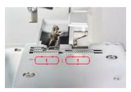
In a default value of 1, the machine achieves optimum sewing results with most applications. The Differential Feed in default setting 1 for flat and even seams.
