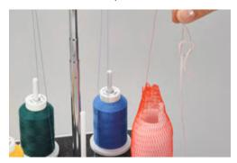
> Pull the end of the thread from the eye of the hook until the knot emerges.
