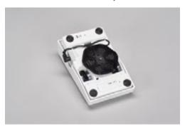
> Insert the cable of the foot control into the foot control connection (1).
