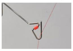
> Engage the thread by pushing downwards into the thread pre-tension with both hands and check by pulling it upwards to the back that it does not slide out of the thread pre-tension.
