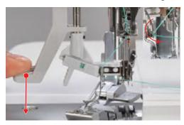
> Release the pressure on the needle threader selector and let it go back to its initial position.
