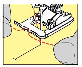
> Pull both cords ends under the buttonhole foot to the front and place each a cord into a groove of the sole.
