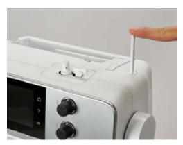
Inserting foam pad and thread spool The foam pad prevents the thread from getting hooked at the retractable spool pin.
