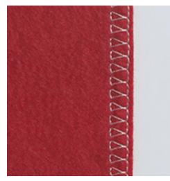
A double overlock seam is suitable for loose knits and cross seams in knits. When working with jersey, a jersey needle should be used to prevent damaging the knit fabric. When sewing stretch materials, use a stretch needle.
