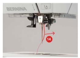
> Pull the thread beneath the attached foot over the thread cutter (15) and cut.
