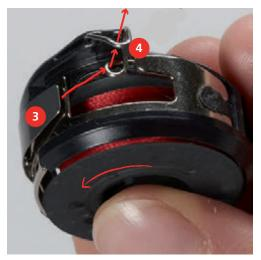
> When inserting into the machine, hold the bobbin case so the the thread guide (5) points upwards.
