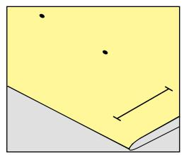
> For keyhole and round buttonholes mark the lenght of the bead with chalk or a water-soluble pen on the fabric. For any subsequent buttonholes mark the starting point. The length of the keyhole is sewn additionally.
