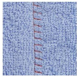
The flat joining seam is especially suitable for or thick materials such as terry cloth, felt and leather.
