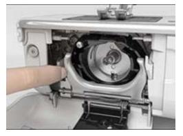
> Flap down the fastening bracket with the black hook race cover.
