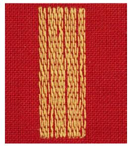
The simple Darning Program No. 22 is especially suitable for quick darning of worn or damaged areas. It is recommended to use fine material as a backing for the worn and damaged areas or to stick an adhesive interlining. The simple Darning Program No. 22 replaces threads along the lengthwise grain in all materials. If the darning area becomes distorted, correct with the balance.
