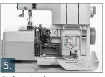
Safety Lockout Prevents the machine from sewing when the front cover is open.
