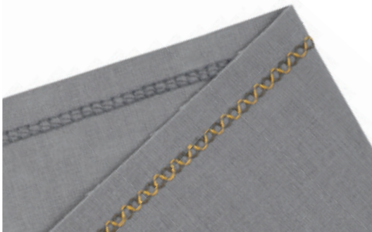
SWING STITCH with double cover stitch - narrow (3 mm)
