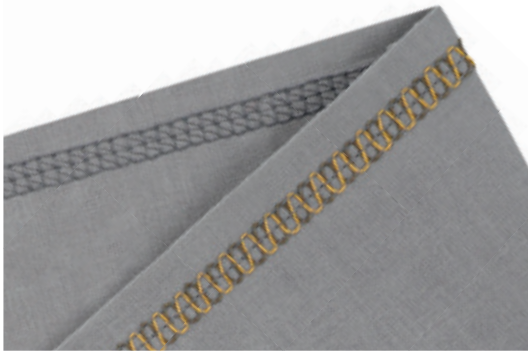
SWING STITCH with triple cover stitch (6 mm)
