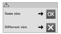
When you stop the machine, a message will appear. Press the OK key and the machine memorizes the seam length to sew another piece of the same length. Press the X key to sew in a different size.
