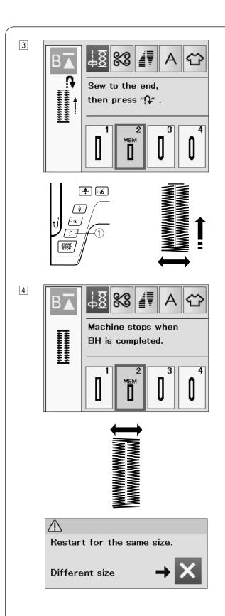
Start sewing again, and the machine sews the front bartack and right side of the buttonhole.Stop the machine when you reach the ending point.
