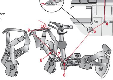
• To thread the last thread guide (9), pull about 10 cm (4") of thread through the guide (8).
