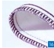
4-thread safety stitch, narrow For joining with reinforced stitch and overcasting in one step.
