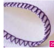
3-thread wrapped overlock wide Perfect for finishing skirts or as lettuce edge on fine fabrics.
