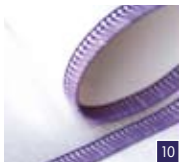
3-thread stretch overlock For sewing extra stretchy light or medium weight fabrics. (Add additional stretch by using a stretchy type thread in the loopers.)
