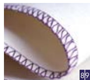
3-thread overlock, wide & narrow Seam, overcast the edge and trim away excess fabric in one step.
