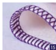
4-thread overlock Seam, overcast the edge and trim away excess fabric in one step. For all seams where stretch or give is needed, such as neck edges, side seams, sleeves.
