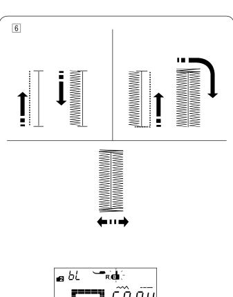
6 The buttonhole is sewn automatically in the sequence shown. When the buttonhole is finished, the machine will stop automatically with the needle in the up position.
