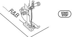
9 Press the start/stop button. The machine will sew "R&B", cut the threads and stop automatically.
